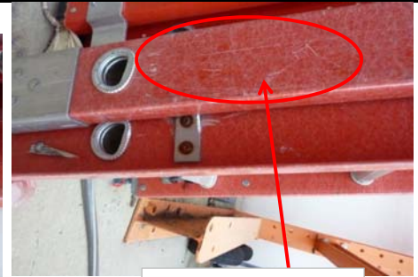
Cracked Fiberglass Rail
