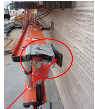
Damaged Safety Shoe : Rubber Pad Damaged
