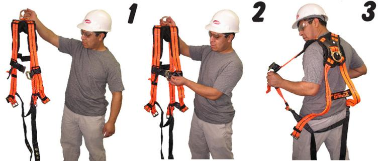
1 Hold the harness by the back dorsal D-ring. Shake harness to allow all straps to fall into place.
