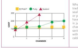
When compared to traditional sleeves sealed with sealant or putty, EZ-Path® will have paid for itself in just three cable changes or less. The savings will increase with each additional cable change.
