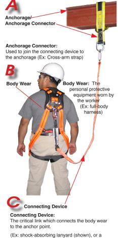
(Ex: shock-absorbing lanyard (shown), or a retractable lifeline)
