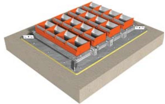
Sturdy steel grids mount one, two or four banks or pathways in built-in slots for a total of up to sixteen pathways through a single floor opening. A single bank Floor Grid comes complete with pathways. Multi-bank Modular Floor Grids are installed with firestop panels sealing each slot. As additional cable capacity is required, firestop panels are removed and pathway modules containing four pathways are installed in each slot.
