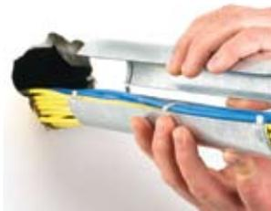
Ready™ Sleeve convenience for existing cable installations. Split sleeve and two-piece wall plates allow sleeve to be assembled around cables and locked into the wall or floor. Available in 1", 2", and 4" sizes.
