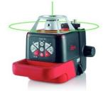
Green beam; motorized mount; receiver/remote control combination
